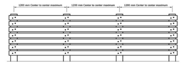
Note: In some cases, the material may be able to span further than local building codes or environmental conditions allow. For example, for an N2 design wind speed, a 600 mm maximum span between supports is recommended. Always consult local building codes and ordinances before starting a project.
