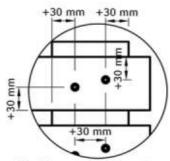
Use 2 screws per connection at least 30 mm from any composite edge
