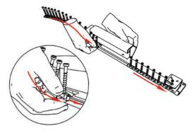
To load a magazine, slide the collation strip into the hand tool via the guide, and then slide the strip to the end of the tool.
